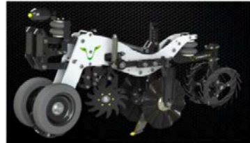
Figure 1. A component of a strip till machine, showing the rakes, ripper tine and press wheel. Image from slyfrance.com
