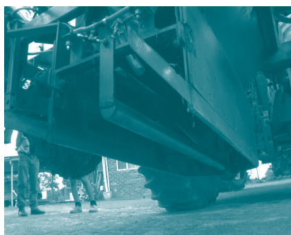
The underside of a "super single" wide throat billet planter
